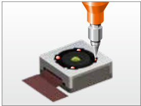
Dispensing UV on Camera Module
