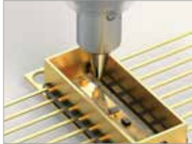
Dispensing Ag Paste on optical communication module
