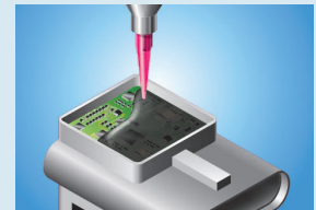
Pressure Sensor Potting
