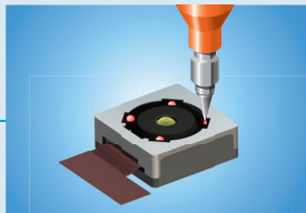
Dispensing UV on Camera Module
